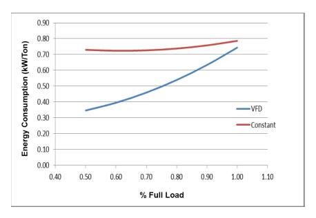
Figure 2: General system differences in efficiency between a constant speed chiller compared with that of a VFD operated chiller.
